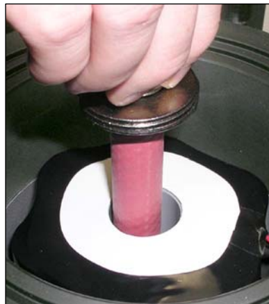
Figure 7C – Inserting battery rod to secure battery pack in main cylinder.
