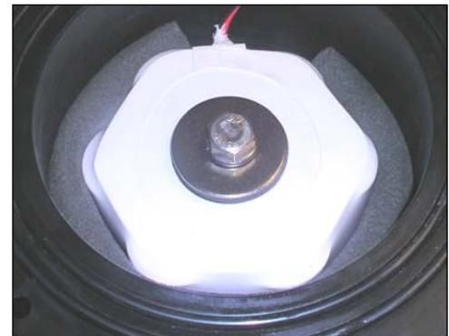
Figure 7D - Foam around circumference of battery pack.
