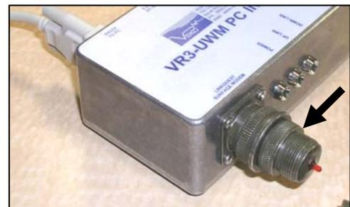
Figure A-4: Interface Loopback connector.
