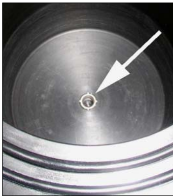
Figure 7B - Battery bolt hole in the bottom of the main cylinder.
