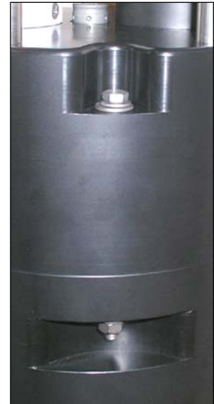
Figure 5 - VR3-UWM halves bolted together.
