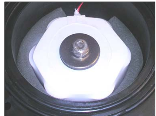
Figure 7D - Foam around circumference of battery pack.
