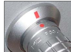
Figure 9 – Power connector in place.
