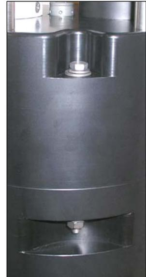
Figure 5 - VR3-UWM halves bolted together.
