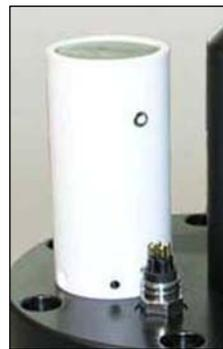
Figure 2 - Bottom modem transducer.
