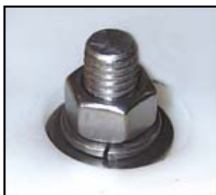
Compressed split washer
