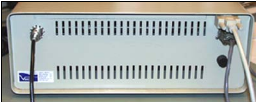
Back panel of Base Station - antenna (left); computer (top right); power (bottom right).
