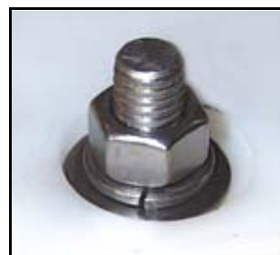
Compressed split washer
