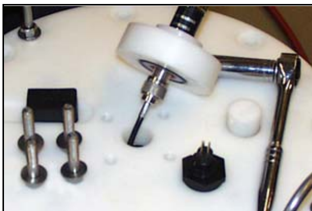
Attaching antenna (bolts and washers are ready)
