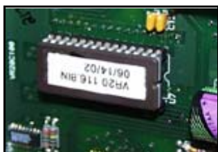
Alignment of new ROM
