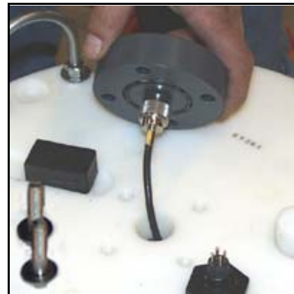
Attaching Antenna Mount Hole Cover (bolts ready)
