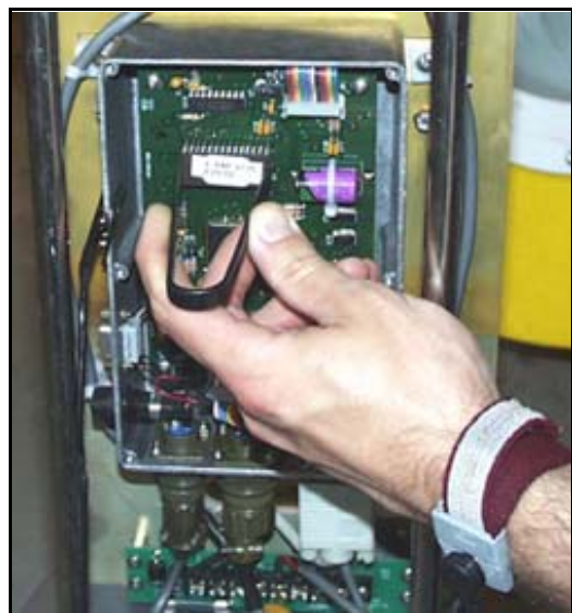
Removing the ROM with the extractor (note the static strap)
