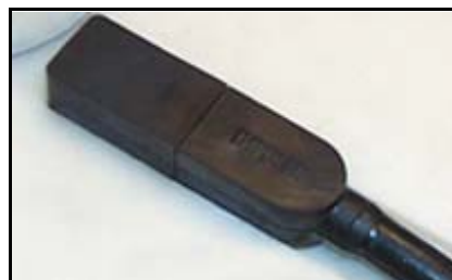
Hydrophone properly connected.
