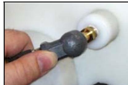
Inserting pressure (air) in the buoy
