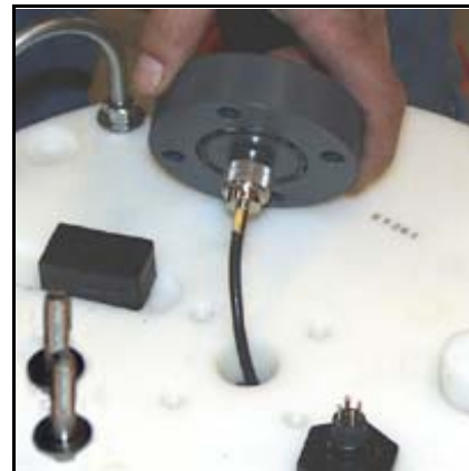
Attaching Antenna Mount Hole Cover (bolts ready)
