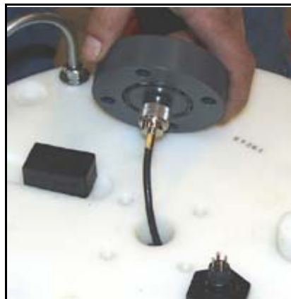
Removing Antenna Mount Hole Cover
