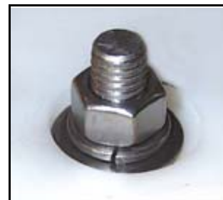
Compressed split washer
