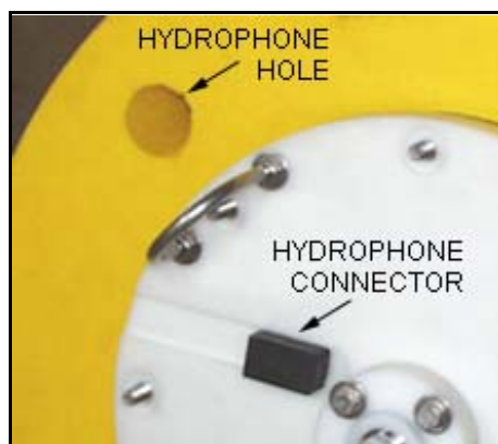
Correctly aligning buoy lid and hull.
