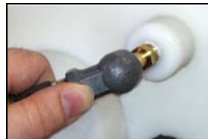
Inserting pressure (air) in the buoy
