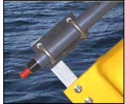
Standard buoy hydrophone in deployed position
