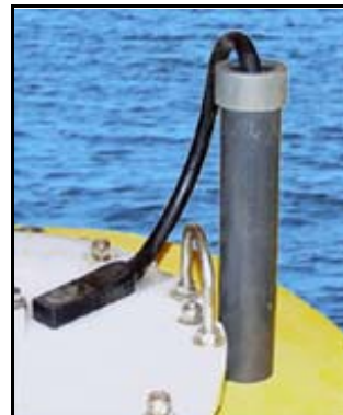
Hydrophone cable when standard hydrophone is in safe position
