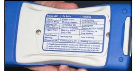
Status LEDs Quick Guide mounted on back of VFR
