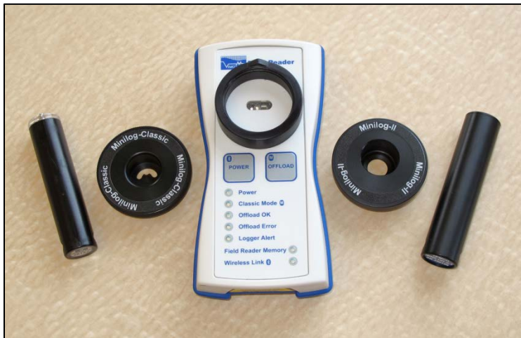
VEMCO Field Reader (center) with the Minilog-Classical and Minilog-II loggers and their adapters.
