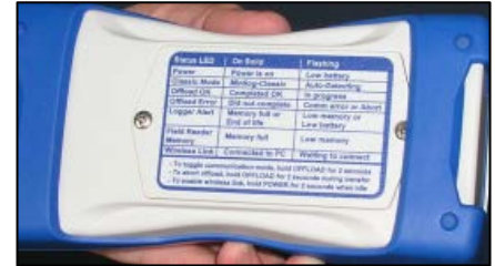
Status LEDs Quick Guide mounted on back of VFR
