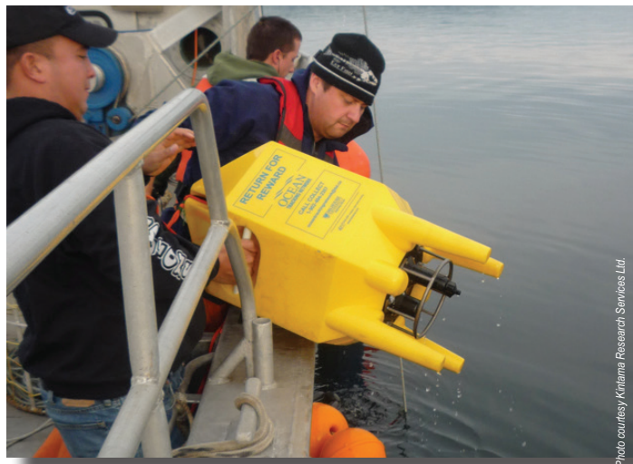
A research team deploys a VEMCO VR4-UWM receiver which is encased in a flotation collar made by Kintama Research.
